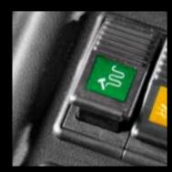
Button for activation of the filter shaking
