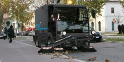
will also find manoeuvring simplified: the brush needs only to be moved to collect waste far from the sweeping machine, while lifting, lowering and rotation are automatic.
